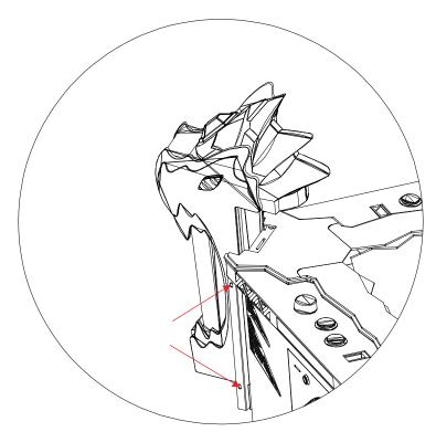
Use 4-M6\*30 screw to the light box on the body (remember to plug in the light wire).
